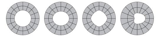
Figure 2: Disk, ellipse with eccentricity 0.5, "generic" domains  $(R = 2 \text{ and } \mathbb{Q}_6 \text{ Meshes})$ .
