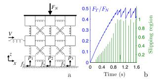
FIG. 1 (color online). (a) Sketch of the 2D spring-block model. (b) Typical loading curve, from static contact to macroscopic stick slip, for setup 1 (h = 5 mm, L = 140 mm,  $F_N = 3500 \text{ N}$ ). Vertical lines: locations of slipping regions for all microslip events. 0 (1) corresponds to the trailing (leading) edge.
