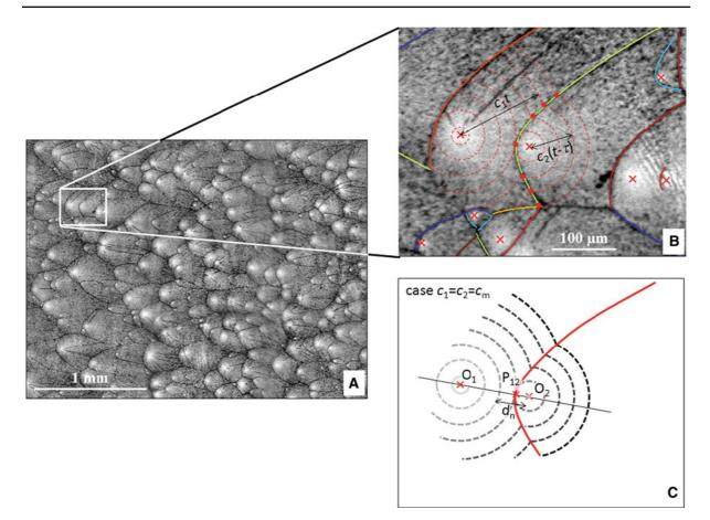
**Fig. 9 a** Typical microscope image of the post-mortem fracture surface. *Bright regions* indicate the nucleation centers. **b** Interpretation of the conic marks: *red dots* sketch the successive positions of the fronts that, by interacting, will be giving rise to the *green branch* of the conic mark. These two microcracks form at t = 0 and  $t = \tau$ , then radially grow at speeds  $c_1$  and  $c_2$ .
