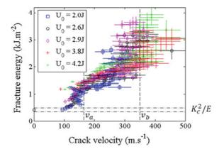
**Fig. 5** Fracture energy  $\Gamma$  as a function of crack velocity v for five different experiments with different stored mechanical energies  $U_0$  at crack initiation. The *two vertical dashed lines* correspond to  $v_a$  and  $v_b$ . The *two horizontal dashed lines* indicate the confidence interval (95%) for the measured fracture energy  $K_c^2/E$  at crack initiation (taken from Scheibert et al. (2010))
