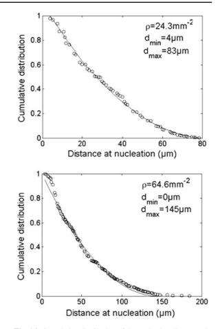
Fig. 16 Cumulative distribution of the nucleation distances  $d_n$ , as measured for two different fractographic images. Solid lines are fits with  $P(d_n) = ((d_{\text{max}} - d_n)/(d_{\text{max}} - d_{\text{min}}))^2$
