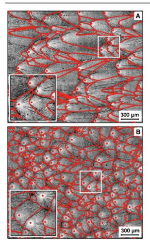
**Fig. 12** Qualification of the procedure: superimposition of the conic pattern as obtained from reconstruction onto that observed by fractography. **a** K = 2.77 MPa  $\sqrt{m}$ . **b** K = 4.18 MPa  $\sqrt{m}$ . *Red dots* indicate nucleation centers (taken from the supporting information of Guerra et al. (2012))
