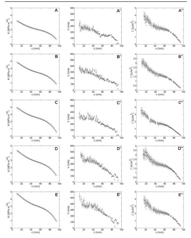
**Fig. 4** Variation of SIF *K* (*left*), instantaneous crack velocity v (*center*) and fracture energy  $\Gamma$  (*right*) as a function of crack length *c* for five experiments with different stored mechanical
