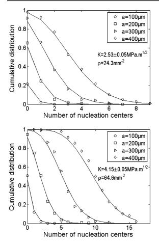
Fig. 14 Cumulative distribution of the number of nucleation centers contained in square regions of lateral size a, for two different fractographic images. *Solid lines* represent Poisson fits of parameter  $\rho a^2$ , where the fitted value  $\rho$  can be identified with the center density
