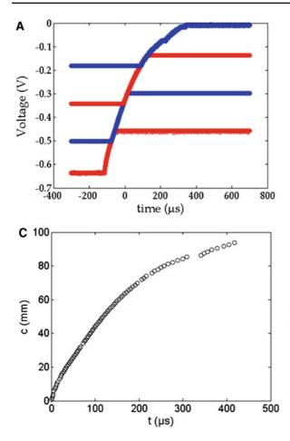
Fig. 2 Measurement of instantaneous crack velocity.  $\mathbf{a}$  Voltage as a function of time as recorded via the oscilloscope.  $\mathbf{b}$  Zoom that permits to distinguish the individual jumps yielded by the
