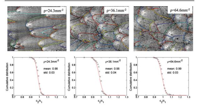
**Fig. 10** Direct extraction of the relative speed between two interacting microcracks at three different microcrack densities. (*Top*) Zones of investigation. Each conic branch has been attributed a given *color* and the nuclei of the two corresponding interacting microcracks has been joined by a *dotted segment* of the *same color*. Note that a conic-like mark is often made of several of these conic branches. The ratio  $c_2/c_1$  is the only adjustable
