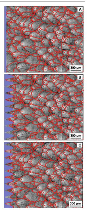
**Fig. 13** Influence of initial crack front morphology on the reconstruction for  $\rho = 45.0 \text{ mm}^{-2}$  ( $K = 3.65 \text{ MPa} \sqrt{m}$ ). Three different initial conditions were used. **a** *Straight vertical line*. **b** *Vertical sinusoidal shape* with a period of 186 µm and a peakto-peak amplitude of 242 µm. **c** *Same sinusoidal shape*, but translated vertically over half a period (taken from the supplementary information of Guerra et al. (2012))
