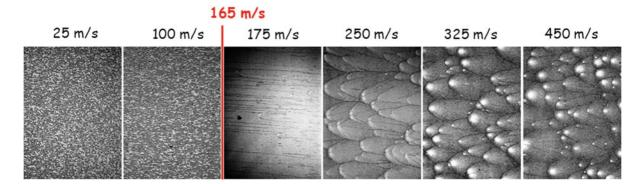
Fig. 6  $1 \times 1.4$  mm<sup>2</sup> microscope images of fracture surfaces created at various speed v
