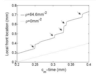
Fig. 21 Position of a given point of the front as a function of "time"  $c_m \times t$  as obtained from the reconstructed simulation, applied to a fracture surface with  $\rho = 64.6 \text{ mm}^{-2}$ . The *dotted straight line* indicates the expected position without microdamage (slope 1). The jumps (*arrows*) correspond to coalescence events with microcracks (taken from Guerra et al. (2012))
