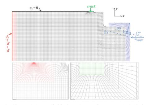
Fig. 3 Computation of SIF. *Top* typical mesh used for finite elements calculations, in order to access the stress/strain fields in the experiments. *Red* polymeric layer. *Black* sample. *Blue* L-shaped block. *Green line* cracked line. The slide link connected to the L-shaped block is used to model the motion of the contact point between the pushed wedge and the roller. Specimen loading is achieved by translating horizontally the slide link, from (0) to
