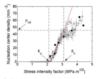
Fig. 15 Variation of the density  $\rho$  of nucleation centers with applied SIF. *Black disks* correspond to the eight images on which post-mortem reconstruction was performed. *Red line* is a fit via Eq. 4.  $K_a$  and  $K_b$  are associated with microcracking and microbranching onset, respectively (taken from Guerra et al. (2012))
