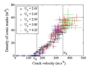
Fig. 8 Surface density  $\rho$  of conic marks as a function of crack velocity for five different experiments with different stored mechanical energies  $U_0$  at crack initiation (taken from Scheibert et al. (2010))
