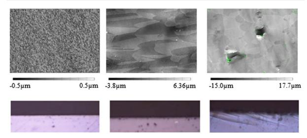
**Fig. 7** Profilometric  $1.4 \times 1 \text{ mm}^2$  surface (*Top*) and optical  $0.7 \times 0.25 \text{ mm}^2$  side-view (*Bottom*) images taken at velocity smaller than  $v_a$  (*left*), between  $v_a$  and  $v_b$  (*center*), and above  $v_b$  (*right*). Crack has propagated from *left* to *right*
