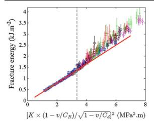
**Fig. 19** Variation of the fracture energy  $\Gamma$  with  $K_d = K \times (1 - v/C_R)/\sqrt{1 - v/C_D}$ . The vertical dashed line corresponds to microcracking onset  $K_d^a = 1.83$  MPa  $\sqrt{m}$ . Note that  $K_d$  can *stricto-senso* be identified with the dynamic SIF in absence of microcracking, *i.e.* for  $K_d \leq K_d^a$ . The *solid red line* is a fit with Eq. 5
