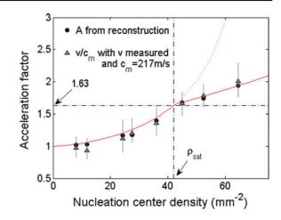
**Fig. 20** Acceleration factor  $A = v/c_m$  as a function of the microcrack density  $\rho$ . *Red line* is a fit by Eq. 9 with  $b = 1.19\pm0.02$ . *Horizontal dot line* defines  $v_b/c_m$  and passes through the slope breakdown observed when  $\rho = \rho_{sat}$  (taken from Guerra et al. (2012))
