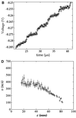
successive cuts of the conductive lines as crack advances. **c** Resulting position of crack tip as a function of time. **d** Final *curve* showing the variations of crack velocity with crack length
