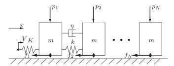
FIG. 1. Schematic of the model system. The slider is modelled as N blocks with mass m connected by springs of stiffness k. The trailing edge block (block 1) is slowly driven through a loading spring of stiffness K. Each block n is also submitted to a normal force  $p_n$ , a friction force  $f_n$ , and a viscous damping force  $F_n^{\eta}$ , which is described by the viscous coefficient  $\eta$ .
