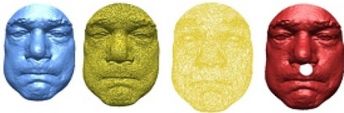
Figure 6: An example of degradations applied to one model. From left to right: the Original face, with Noise, Decimation, and Holes
