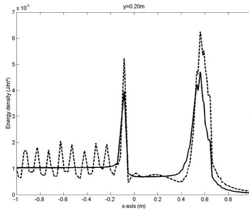
Figure 3: Energy density in linear scale with the radiosity method (-) and with the GTD(- -). Frequency : 2500 Hz.
