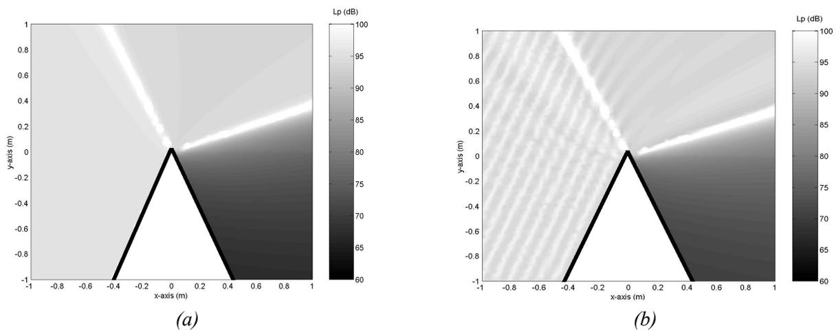
Figure 2: Sound pressure level ( $L_p$ ) in dB with the radiosity method (a) and with the GTD. Frequency : 2500 Hz.
