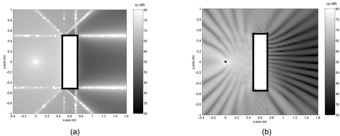
Figure 4: Sound pressure level ( $L_p$ ) in dB with the radiosity method (a) and with the Boundary Element Method (Sysnoise ©). Frequency : 2500 Hz.
