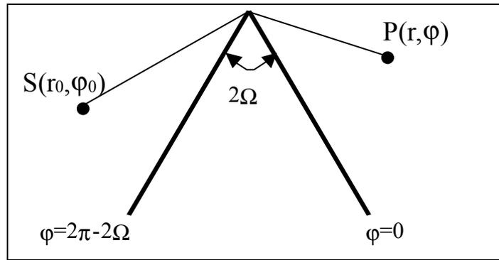
Figure 1: Source and observation point positions
