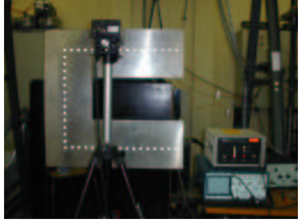
Figure 2: Experiment on a U-shaped plate. View of the experimental setup including the velocimeter and positions of measurement points along a line.
