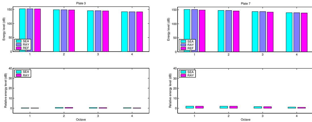
Fig. 2. Vibrational response of plates 3 and 4. for damping loss factor  $\eta=0.1\%$ . Comparison between SEA, uncorrelated rays (RAY) and reference calculation (REF) for the four octave bands from 1 kHz to 8 kHz. The errors between SEA/REF and REF in dB are shown in the bottom bar diagrams.
