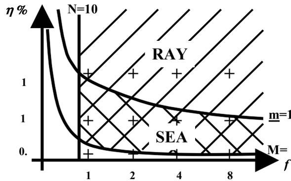
Fig. 5. Validity domain of SEA and uncorrelated rays in the frequency – damping loss factor plane. (\\), SEA domain defined by  $N \gg 1$ ,  $M > 1$ , and  $\underline{m} < 1$ . (//), Ray domain defined by  $N \gg 1$  and  $M > 1$ . (+), position of the twelve calculations of Figs. 2, 3, 4.
