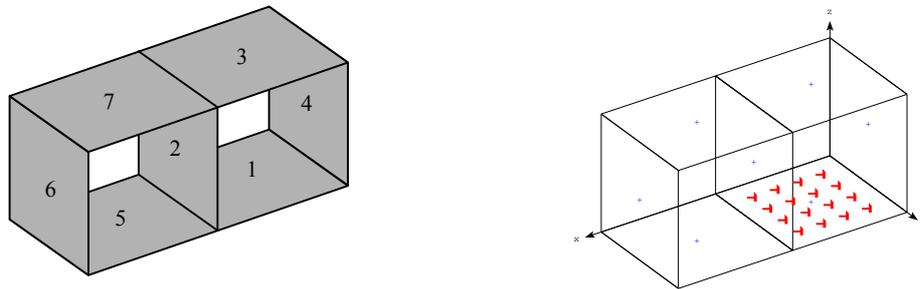
Fig. 1. The seven plate structure. Driving points (small hammers) and receiver points (+).
