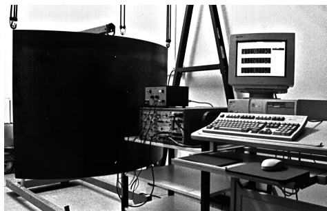
Figure 5: LEA predictions in comparison with experimental results : Upper figure show the mock-up of the car roof constituted from 7 plates with the experimental set-up . The lower figures give comparisons between (o) local energy predictions and (*) measurements.
